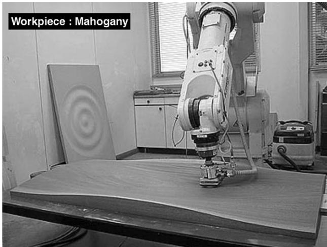
Fig. 15. Sanding scene of wooden table with curved surface.
