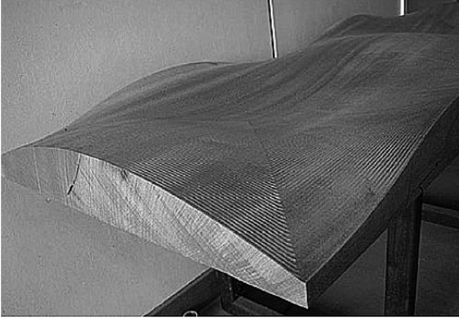
Fig. 12. An example of curved workpiece that conventional sanding machines cannot deal with.
