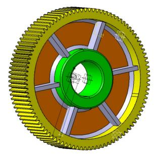
Figure 5: Cylindrical gear made by welding
