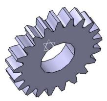
Figure 3: Simplest model of cylindrical gear
