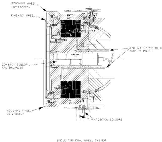
Fig. 5. Single axis dual wheel system.
