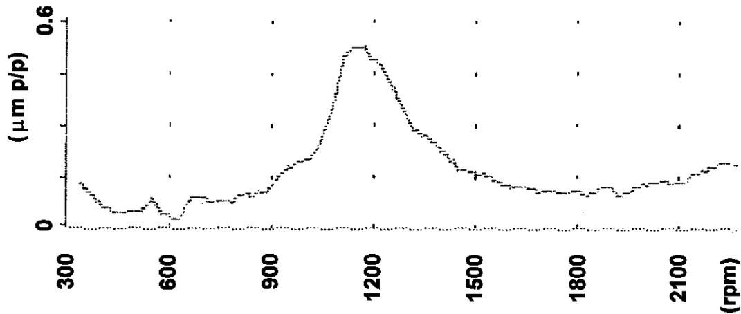
Fig. 6. Grinding spindle – horizontal amplitude response to out-of-balance forces.
