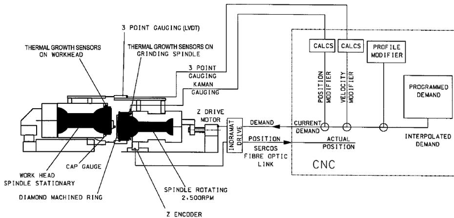
Fig. 4. Z-axis functional block diagram.
