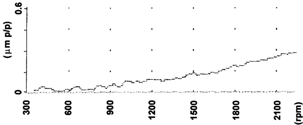
Fig. 8. Grinding spindle – vertical amplitude response to out-of-balance forces.
