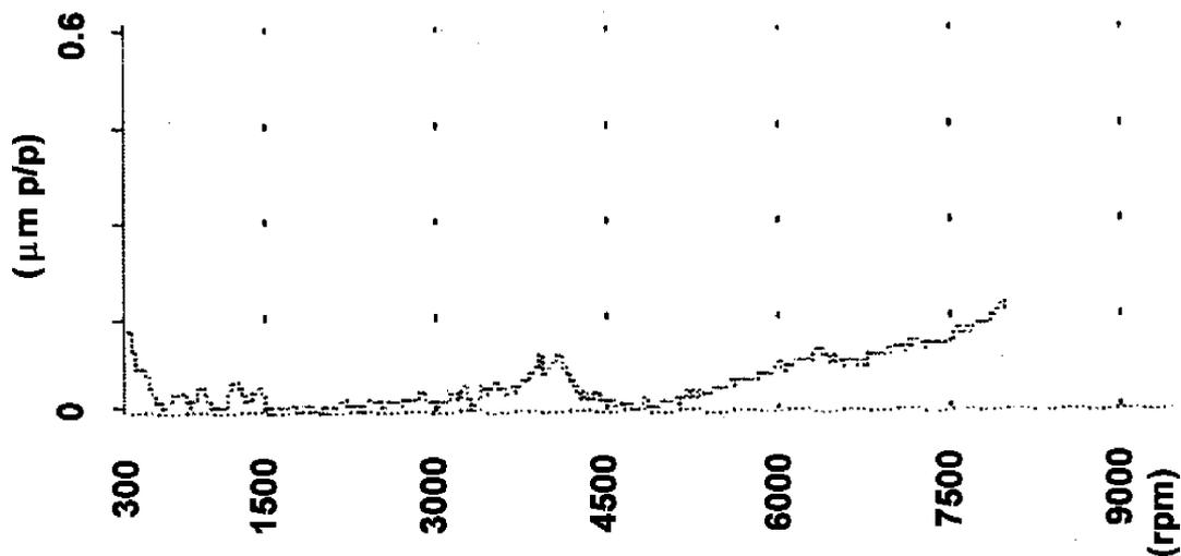
Fig. 9. Truing spindle – horizontal amplitude response to out-of-balance forces.
