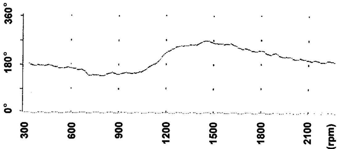
Fig. 7. Grinding spindle – horizontal phase response to out-of-balance forces.
