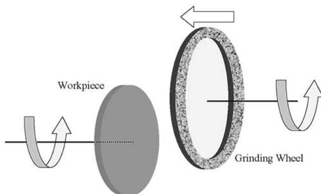
Fig. 1. Face grinding operation.
