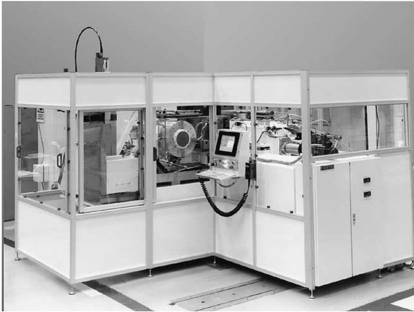
Fig. 2. Face grinding machine.
