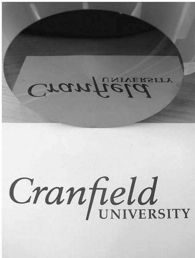
Fig. 10. 200 mm wafer as finish ground – 15 nm Ra.
